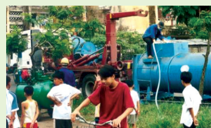
Photo 10: Intermediate storage tank located in the nearest accessible road. (Sandec, 2002, Hai Phong, Vietnam)
