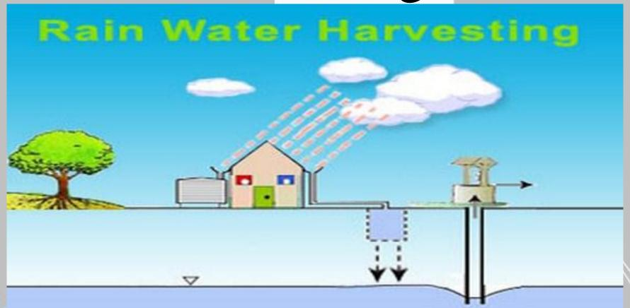
An artificial process of collecting and capturing rainfall, close to where it falls and using it with minimum loss or wastage, close to where it falls. The rainwater can be directly used by storing into tanks or can be recharged into groundwater
