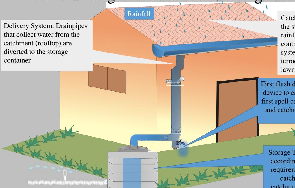
Catchment: The catchment is the surface which receives rainfall directly and contributes the water to the system, e.g: paved area like terrace. Or unpaved area like lawn or open ground
