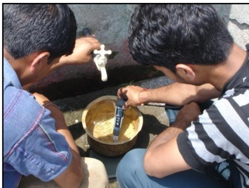
Water quality measurement using a pocket tester
