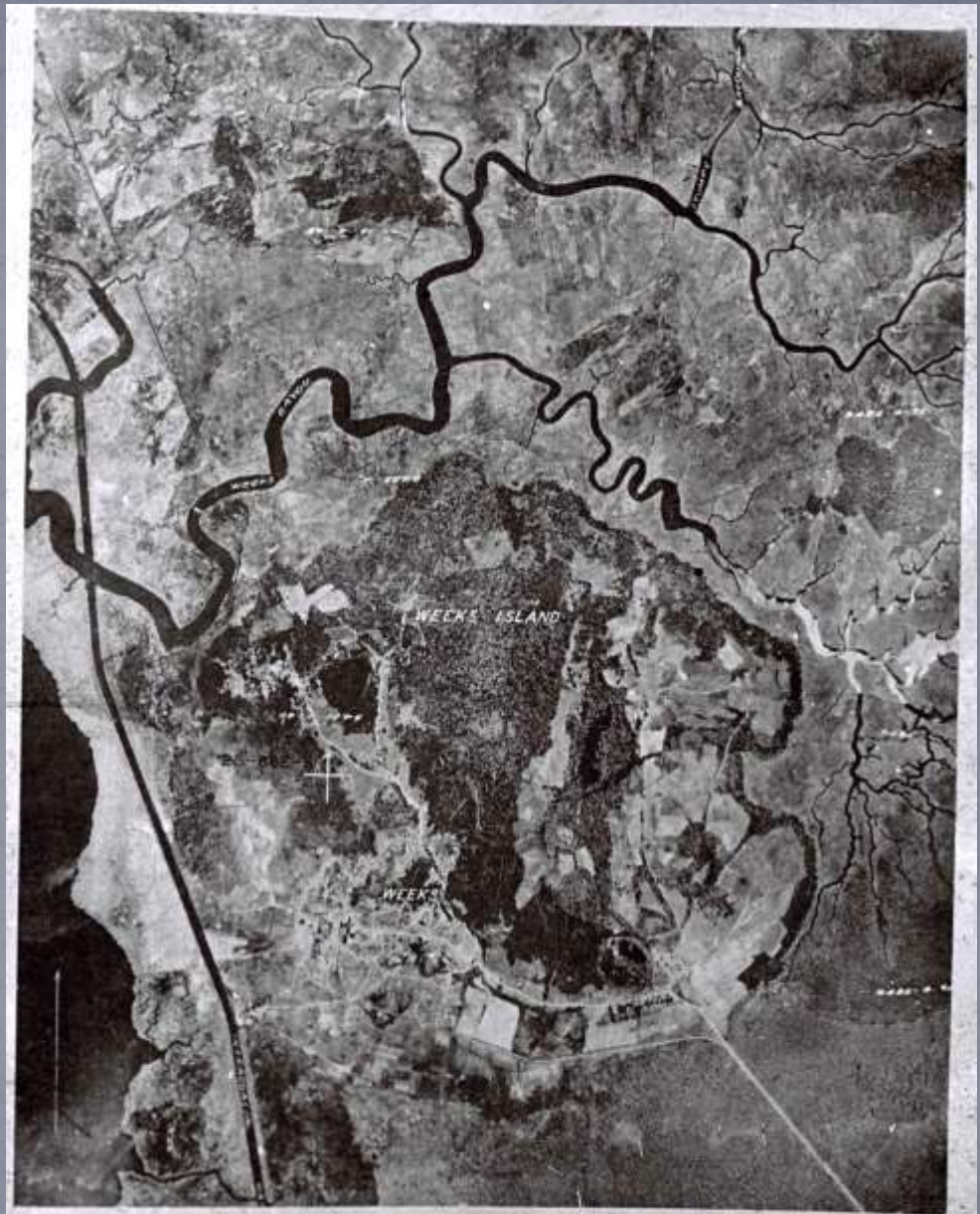
Figure 12-1. Mosaic of a circular topographic high directly underlain by a salt dome. The surrounding area is a lowland coastal swamp. (By permission from Edgar Tobin Agriol Resources.)
