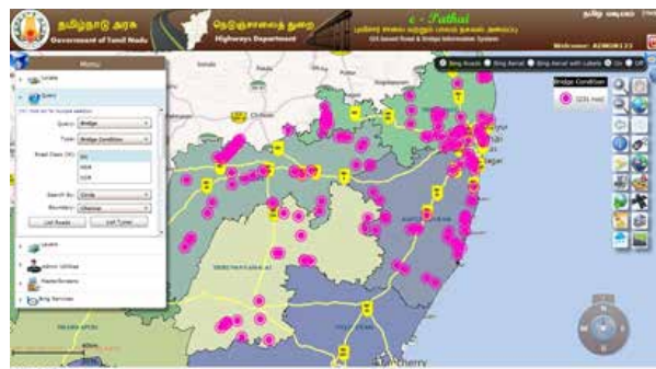
Figure: 4 Thematic for Query on Bridge Condition
