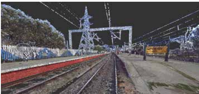
Figure 1: Scan data acquired by the FARO Laser Scanner Focus 3D X 330.
