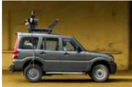
Figure 2: Mobile LiDAR Mapping System
