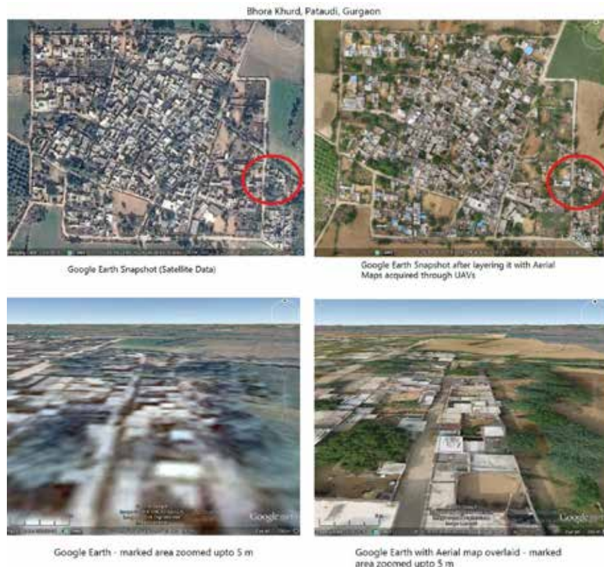
Figure 1: Ground images obtained through UAVs reveal on-ground nuances in comparison to satellite images
