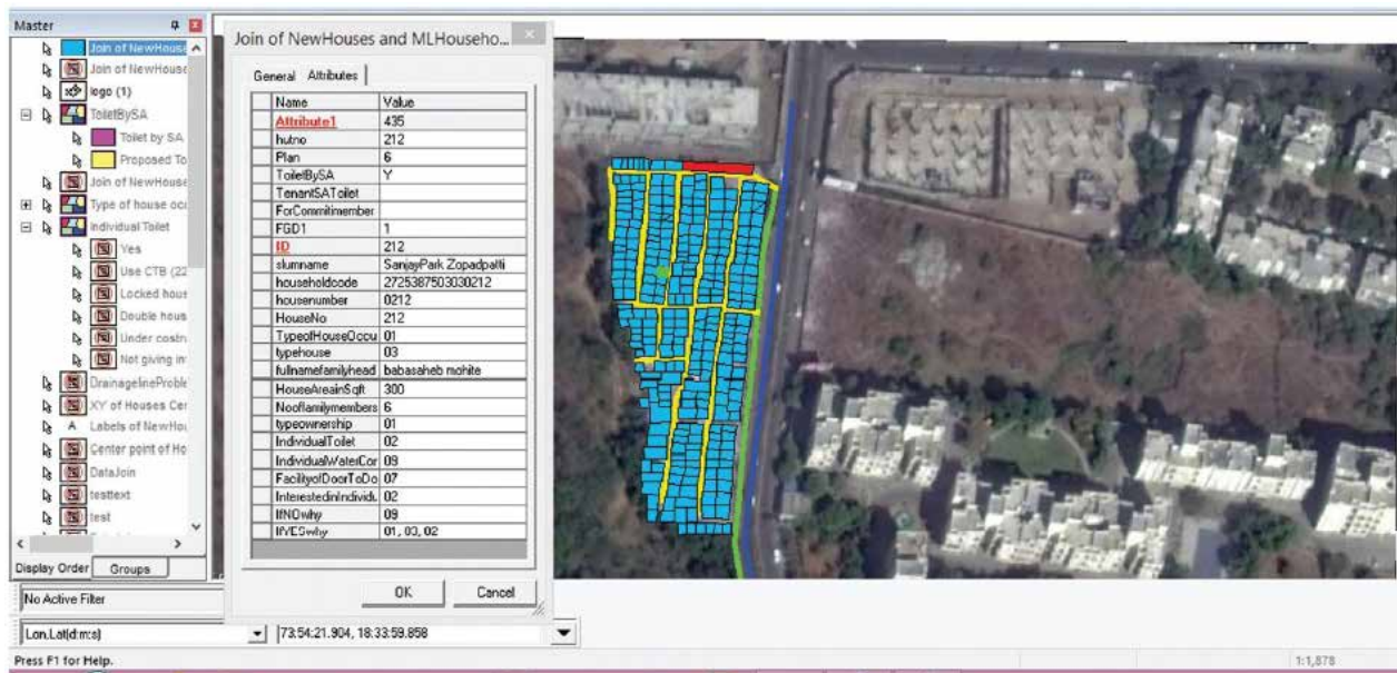
Figure 2: Linking household data (left) to maps (right) results in a comprehensive summary of each household and its occupants
