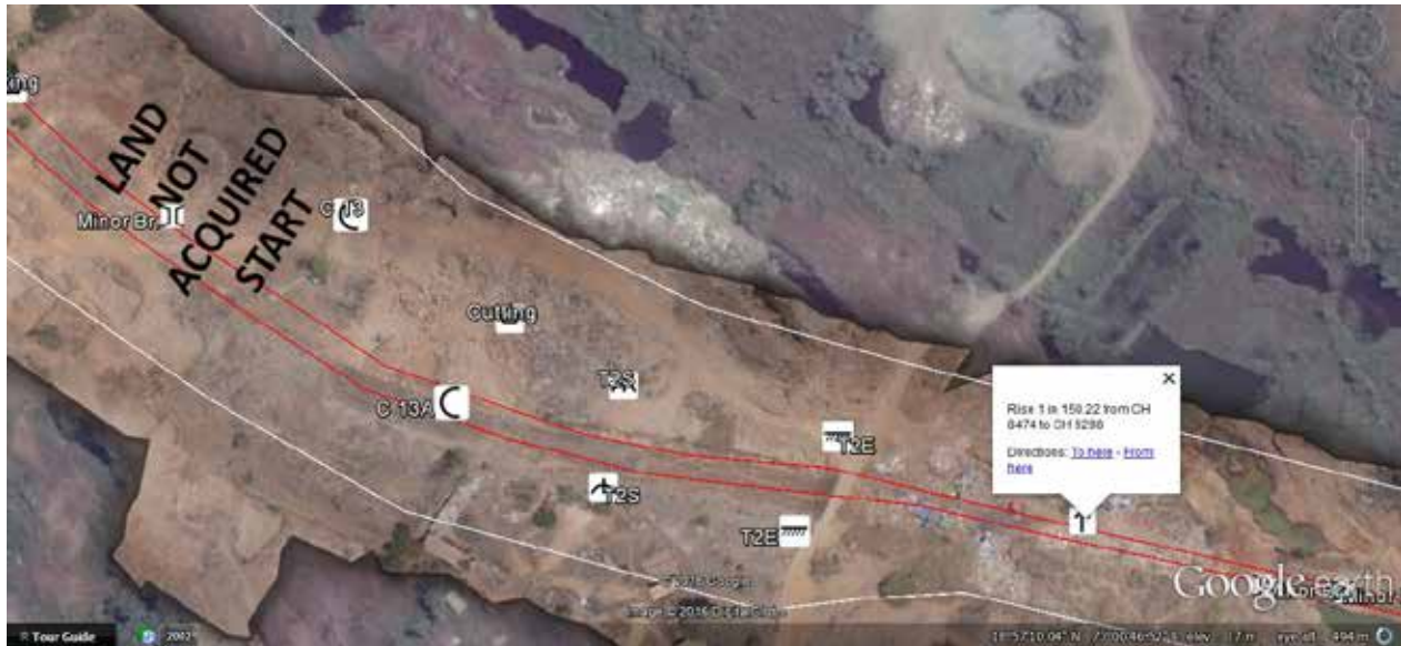
Figure 5: Screenshot of Google Earth file with design data overlay on base layer of processed aerial data
