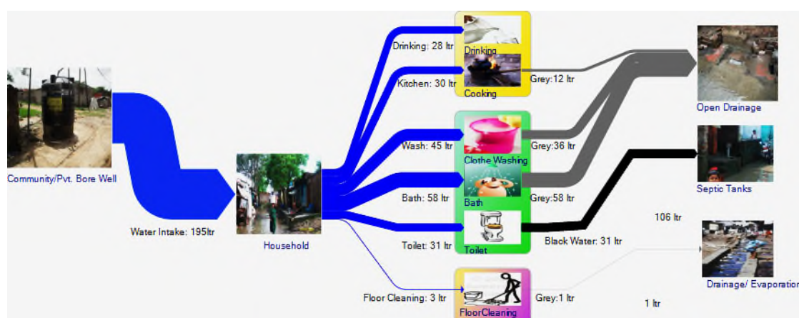
Figure 17: Sankey diagram of water use : of low SEC family
