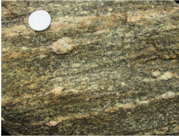
Fig. 6: Mylonites representing shear zone exposed at the landslide plane
