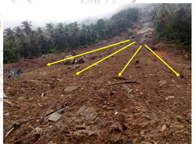
Fig. 5: Flow chutes through which debris material flown
