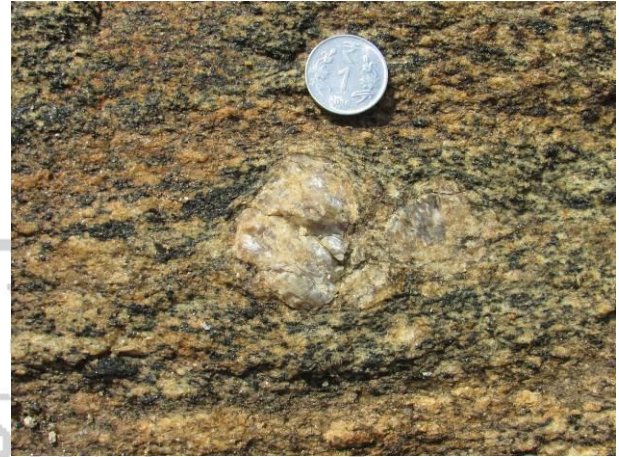
Fig. 6: Mylonites representing shear zone exposed at the landslide plane
