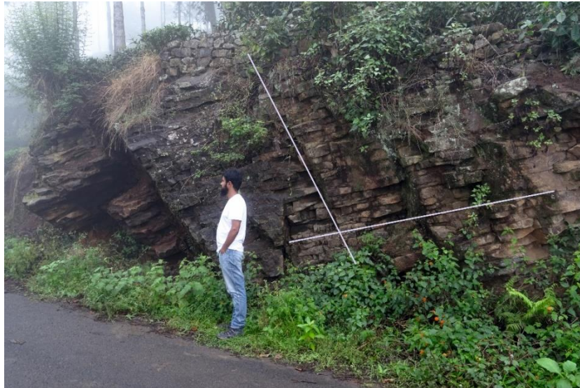
Photo 2: A charnockite or gneiss roadside outcrop showing two sets of fractures; several nearly horizontal and a few high angle dipping fractures
