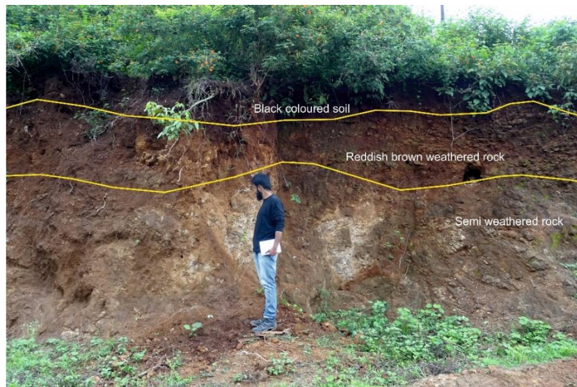
Photo 4: A cross sectional profile revealing the different degrees of weathering - top black coloured soil underlain by reddish-brown weathered rock which overlies a semi-weathered rock
