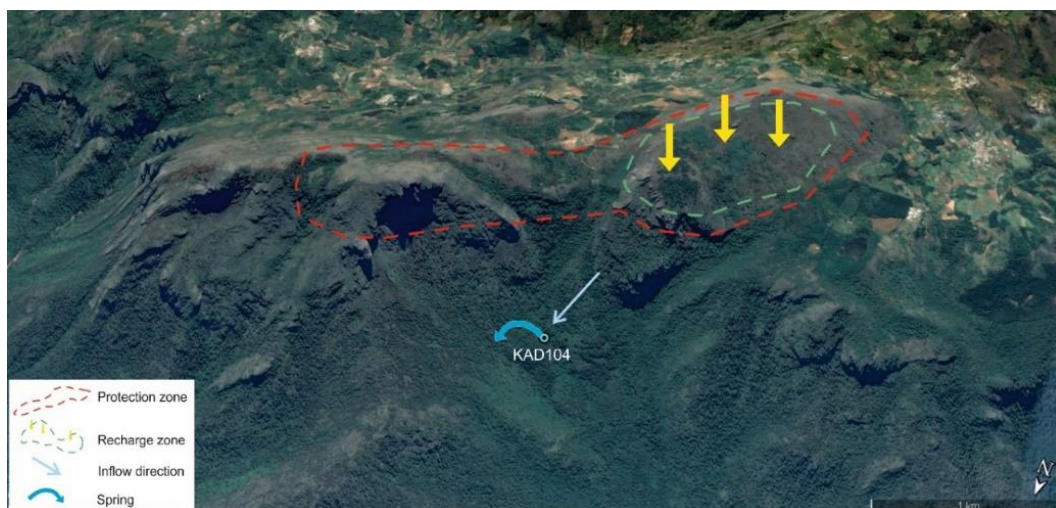
Figure 13: Google earth image showing the protection and recharge area of a spring near Chokkanalli village, Aracode
